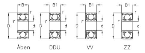
Max rpm ZZ-WW = 40000В = 5 В1 = 5 r min = 0.2Type d = 6 = 696D = 15 Load Cor (N) = 670Load Cr (N) = 1730 Max rpm DD = 36000Max rpm open = 45000
